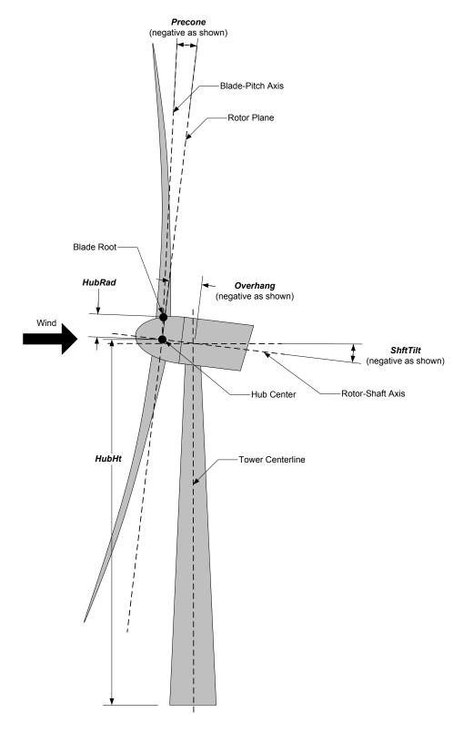
Figure 1. AeroDyn Driver Turbine Geometry
