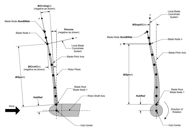
Figure 3. AeroDyn Blade Geometry – Left: Side View; Right: Front View (Looking Downwind)
