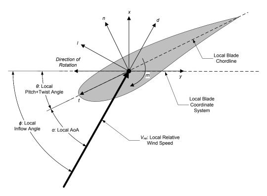
Figure 4. AeroDyn Local Blade Coordinate System (Looking Toward the Tip, from the Root) – *I*: Lift, *d*: Drag, *m*: Pitching, *x*: Normal (to Plane), *y*: Tangential (to Plane), *n*: Normal (to Chord), and *t*: Tangential (to Chord)
