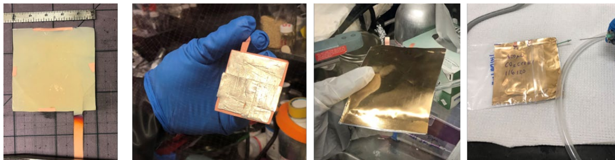
Figure II.1.B.72. Images of the Si electrode (left), Li electrode (center left), pouch cell being injected with electrolyte (center right) and pouch cell injected with CO 2 (right).
