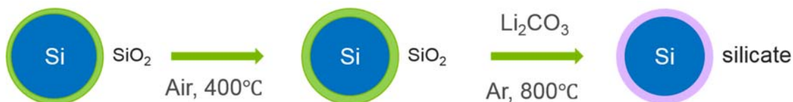
Figure 1 Diagram for the synthesis of Li 2 SiO 3 -coated silicon nanoparticles
