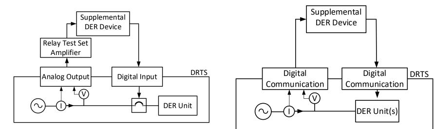
Using a Controller HIL-test setup to confirm operation of supplemental DER devices
