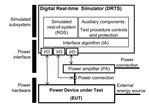
Power Hardware-in-the-Loop test setup overview
