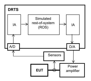
Interface algorithm linking simulated ROS with power amplifier and EUT
