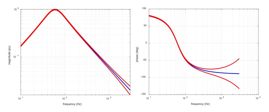
• Magnitude requirement: for  $f_{LL} \le f \le f_{UL}$  the impedance magnitude |Z| shall be within a magnitude range  $|\Delta Z|$  about the simulated RLC-load with  $|\Delta Z| = \max(2.5\%, 2.5\% + (f - 60Hz) / f_{UL} * 30\%).$
