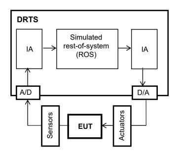
Interfacing EUT to the simulated ROS in a CHIL test setup
