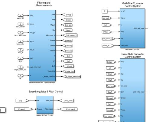
Wind Turbine controls - GE DFIG 1.5MW
