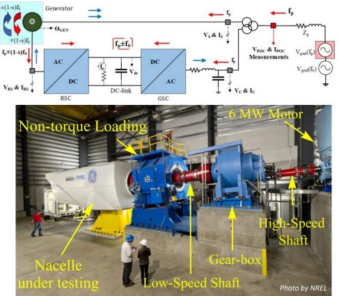
Figure 3.3: Grid and wind/torque emulators at NREL [12]
