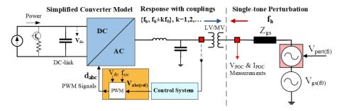
Figure 3.1: Typical example of a grid-connected converter and state-of-the-art form of couplings in response to a single perturbation.
