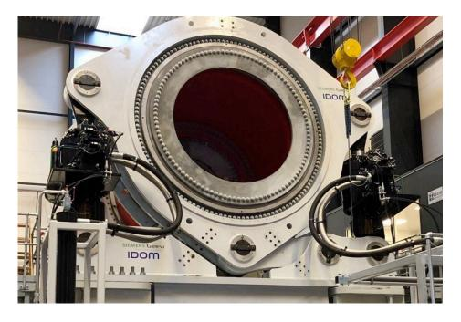
LOAD APPLICATION SYSTEM FOR MAIN BEARING TEST BENCH CLIENT: SIEMENS GAMESA SCOPE: EPC COUNTRY: DENMARK
