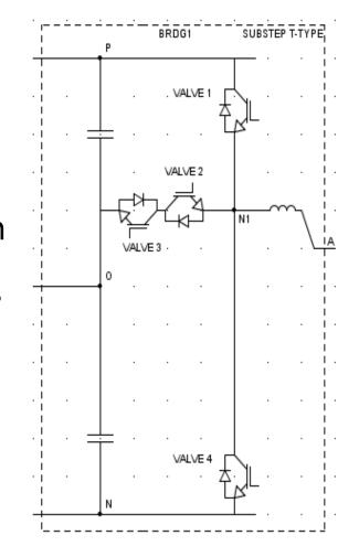
T-type resistive switching model
