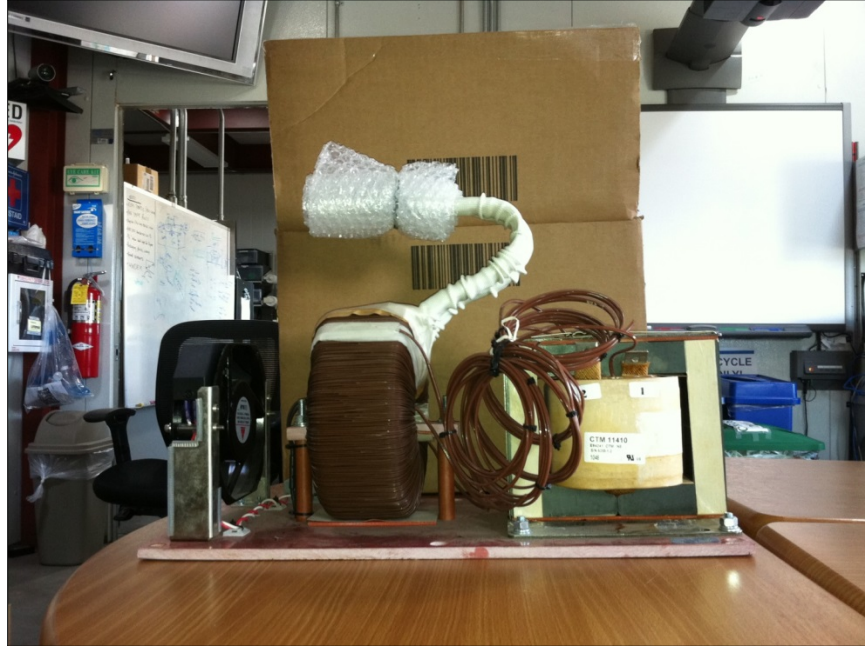
Figure 4. Prototype HFX and resonant inductor. Photo by Mariko Shirazi, NREL
