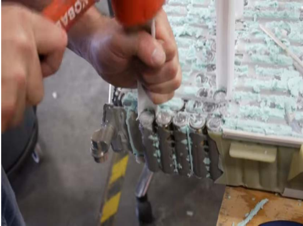
Figure 4. Pack disassembly—thermoplastic materials challenges.
