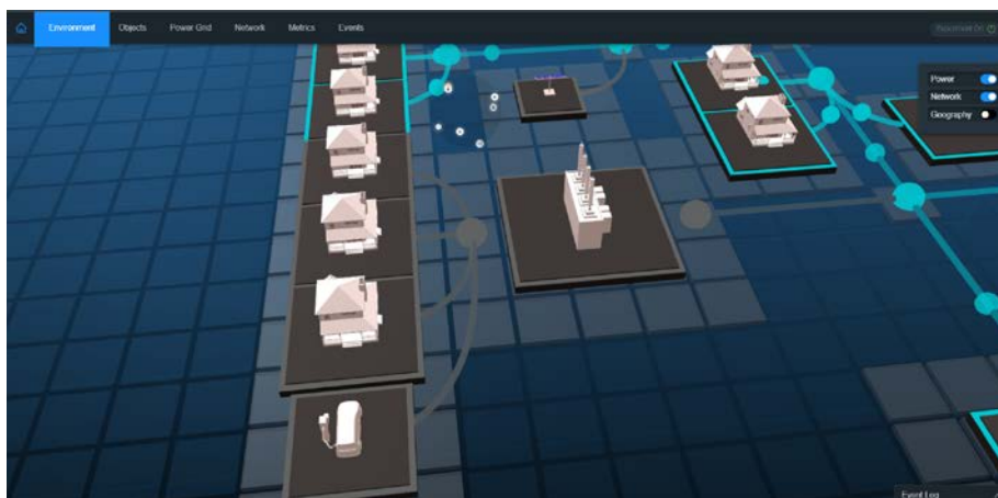
Figure 17. The substation power-off after an MITM attack
