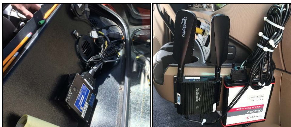
Figure 1. ISAAC data logger (left) and Vector GL2000 data logger (right).
