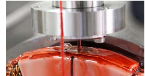
ATF jet impingement on a heated target. Photo by Bidzina Kekelia (NREL)
