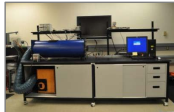
Air cooling loops
