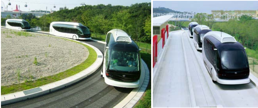
Figure 6. Toyota first demonstrated platooning of AV technology in the Aichi Expo (left), with the off-line station concept shown on the right.
