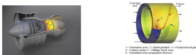
Figure 2: (a) A conceptual rotating detonation turbojet engine [1] (b) The combustion chamber of a Rotating Detonation Engine (RDE) [1]
