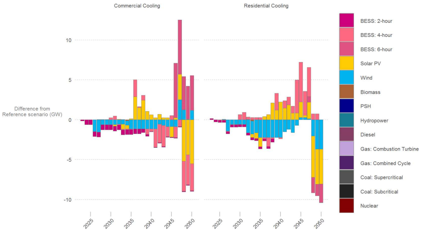
Figure 15. Increased Cooling Load scenarios: Difference in installed capacity of generation technologies compared to Reference scenario
