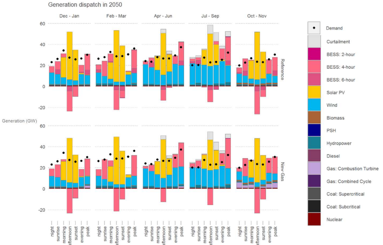
Figure 10. Reference versus New Gas scenario: Generation dispatch and demand in Karnataka for time-slices and seasons in 2050
