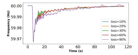
Figure ES-3. Homogeneous packet loss with different loss rates
