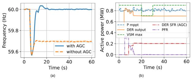
Figure 14. (a) Frequency response with/without AGC and (b) DER power output, PFR, SFR, and its MPPT and VSM limits
