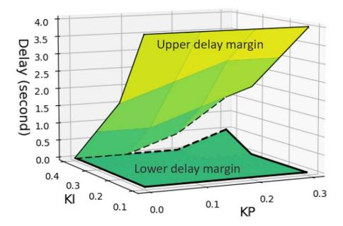
Figure 24. Feasible space of the three values in turbine governor AGC controls
