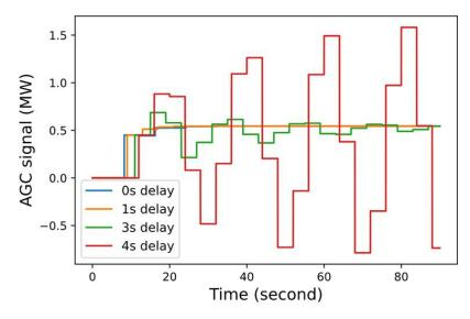
Figure 22. DER AGC signals under different communication delays
