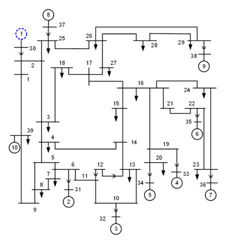
Figure 20. IEEE 39-bus transmission test system
