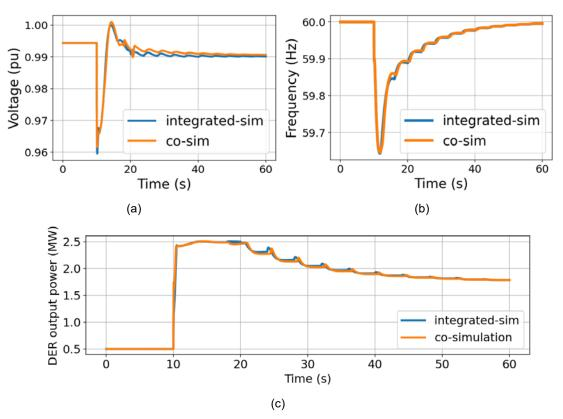
Figure 10. Comparison of the integrated T&D network simulation and the proposed co-simulation: (a) voltage response, (b) system frequency response, and (c) DER power output under the generation drop case
