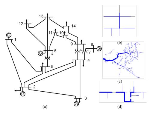
Figure 9. Integrated T&D network with IEEE 14-bus system: (a) IEEE 14-bus transmission system, (b) IEEE 13-bus feeder used for validation, (c) IEEE 8,500-node feeder, and (d) IEEE 34-bus feeder
