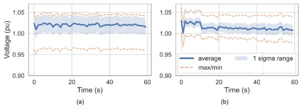
Figure 13. Voltage plots of (a) 34-node feeder and (b) 8,500-node feeder
