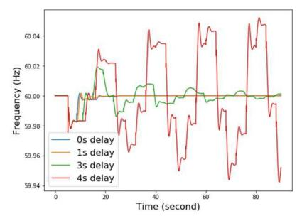
Figure 21. System frequency response under different DER delay signals
