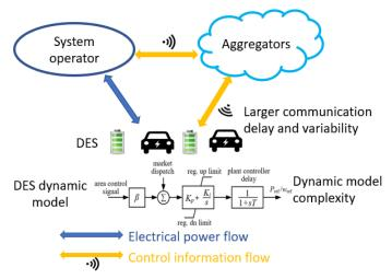
Figure ES-1. Illustration of the DER CPDS model for the provision of reliable frequency regulation services
