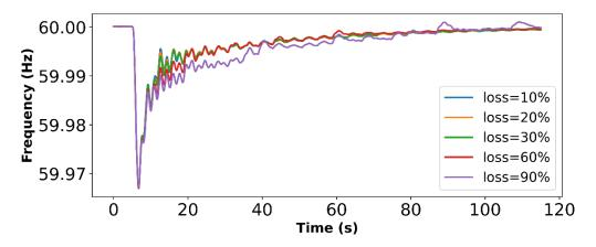
Figure 39. Homogeneous packet loss with different loss rates
