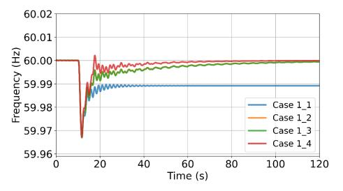
Figure 27. System frequency response under different scenarios
