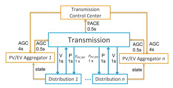
Figure 26. Simulation components with information exchange for the transmission-distributioncommunication system
