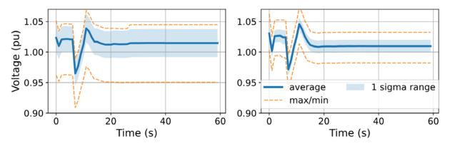
Figure 15. Voltage response of (a) 34-bus feeder and (b) 8,500-node feeder
