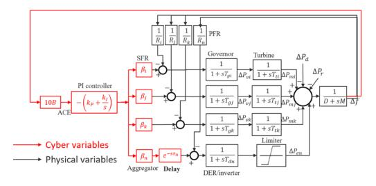
Figure 18. Schematic model of the cyber variables (red) with delays and the physical parts in the transmission system (black)
