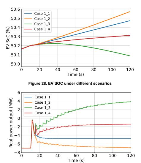
Figure 29. EV real power output under different scenarios
