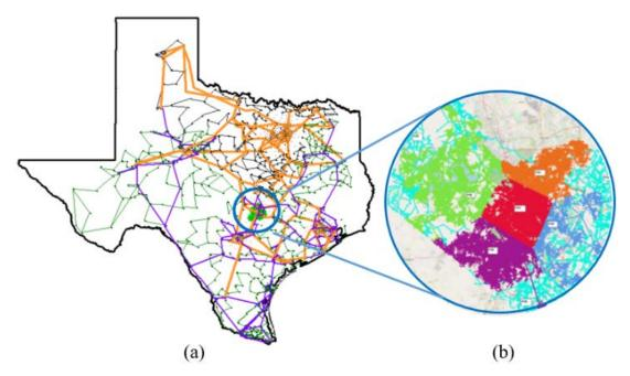
Figure 16. (a) One-line diagram of the 2,000-bus case [60], with the Austin area marked in green, and (b) five subregions in the distribution Austin data set [65]
