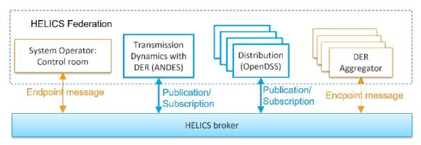
Figure 5. Co-simulation framework structure in HELICS
