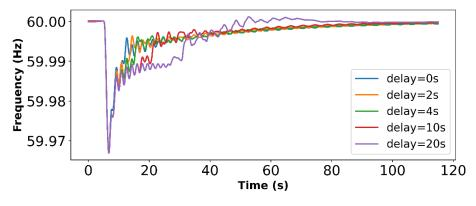
Figure 34. Homogeneous delay with different delay times
