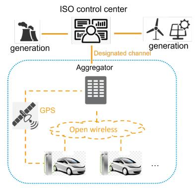
Figure 3. Typical LFC system with EV aggregators
