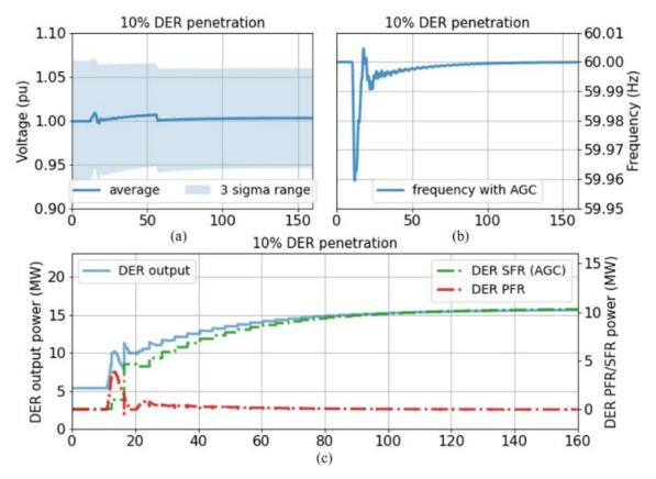
Figure 17. Representative co-simulation results of the 2,000-bus case: (a) voltage profiles of a substation bus connected with distribution feeders; (b) system frequency response; and (c) DER power output, PFR, and SFR
