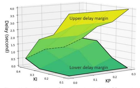
Figure 23. Feasible space of the three values in DER AGC controls
