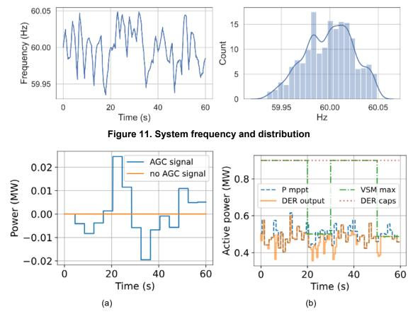
Figure 12. (a) Example of one DER AGC signal from a DER aggregator and (b) example of the power output from one DER under the load variation
