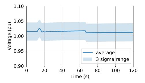
Figure 33. Case Pcap = 1, voltage of substation Bus 6032 with all downstream feeders, with medium-voltage and low-voltage nodes
