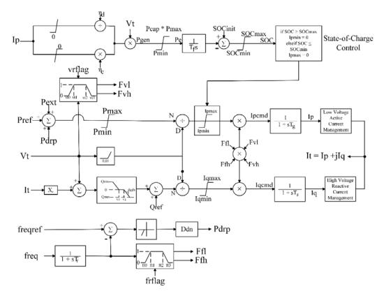
Figure 25. Block diagram for EV dynamic model including PFR
