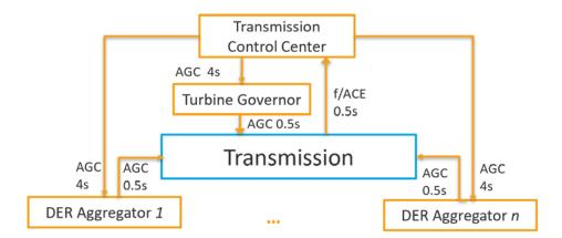
Figure 19. Simulation components with information exchange
