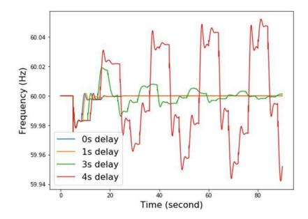
Figure ES-2. System frequency response under different delays
