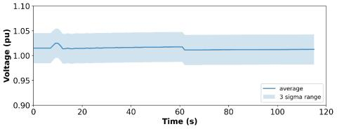
Figure 37. Distribution bus voltage example: the average and 3-sigma range of the voltages among all medium-voltage nodes
