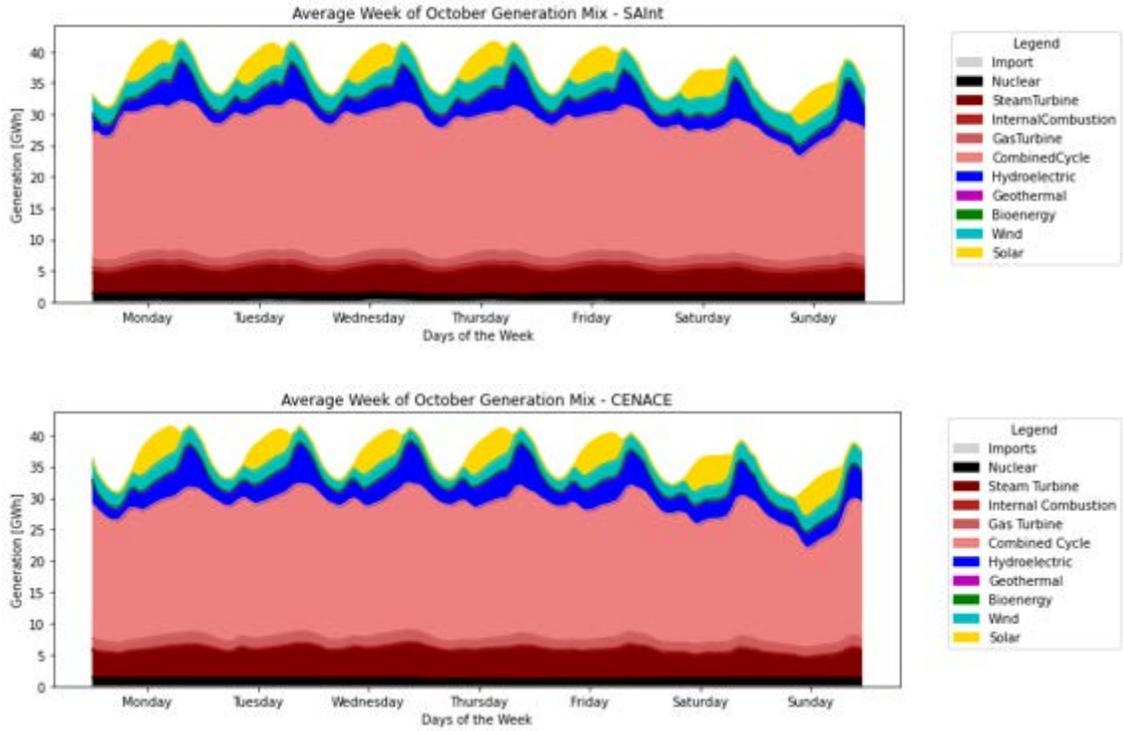
**Figure A-4. Average Weekly Dispatch Per Generation Technology for October**
