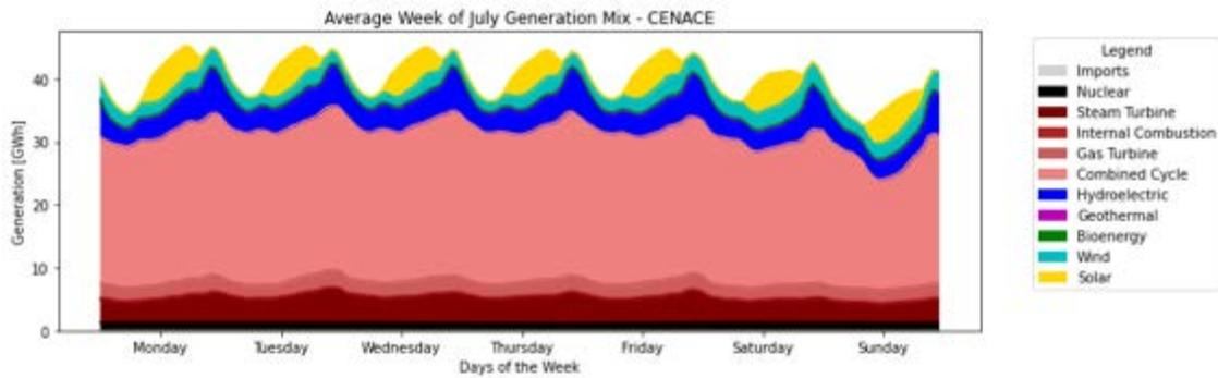
Figure A-3. Average Weekly Dispatch Per Generation Technology for July
