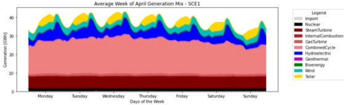
Figure B-22. Average weekly dispatch for each generation technology in April: Scenario 1
