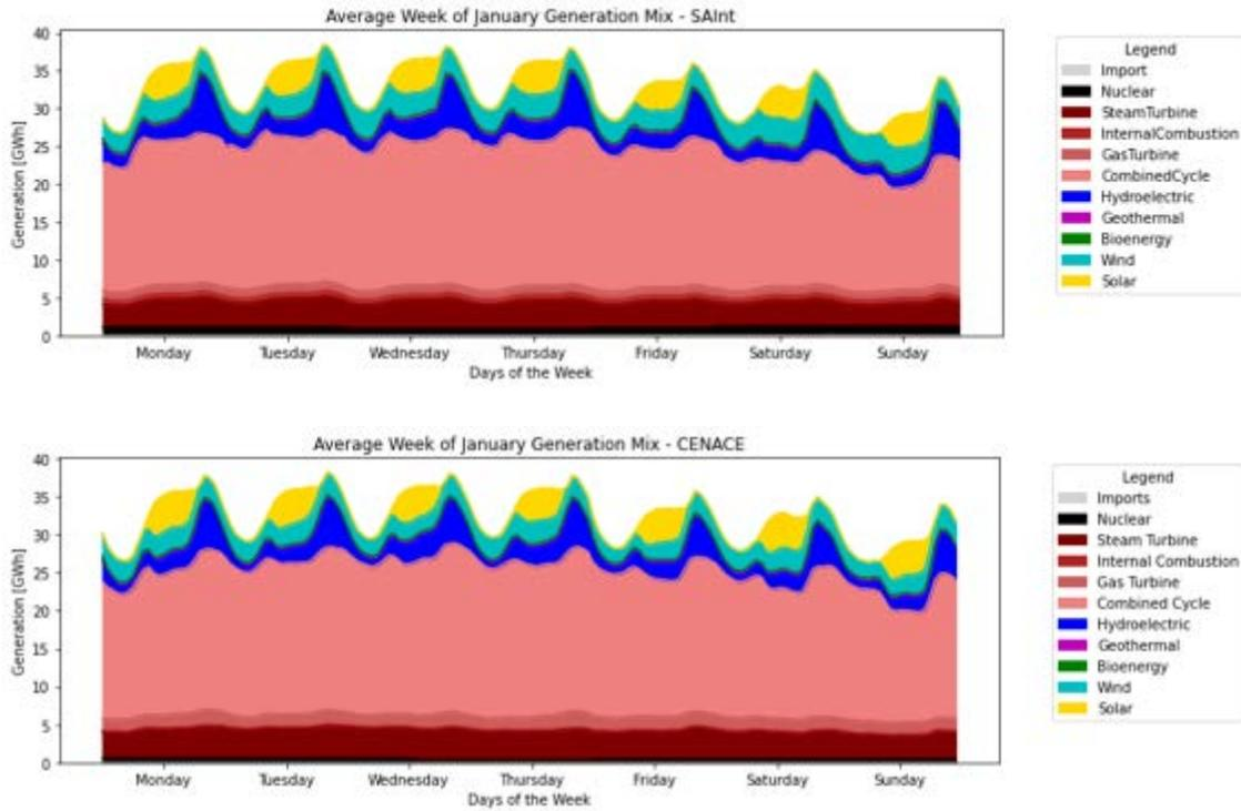
**Figure A-1. Average Weekly Dispatch Per Generation Technology for January**
