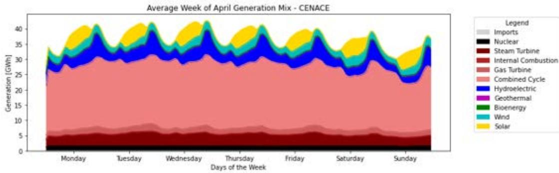
Figure A-2. Average Weekly Dispatch Per Generation Technology for April
