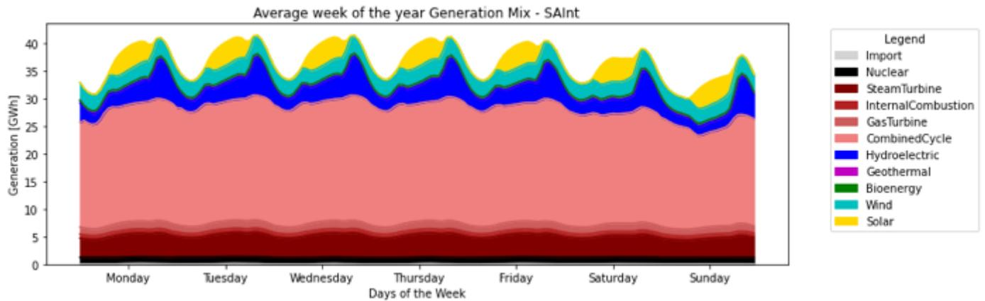
**Figure 15. Average weekly generation dispatch: SAInt modeling outputs**
