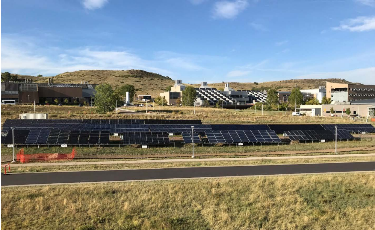
Figure 1. Overview of the NREL PV Lifetime field samples ca 2018
