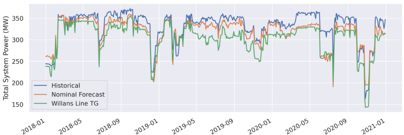
Figure 6. Total system power generation, comparing historically measured data versus the nominal forecast model (including the turbine generator multi-linear regression model) and the Willans Line turbine generator forecast (using a constant value for turbine generator steam consumption rate).
