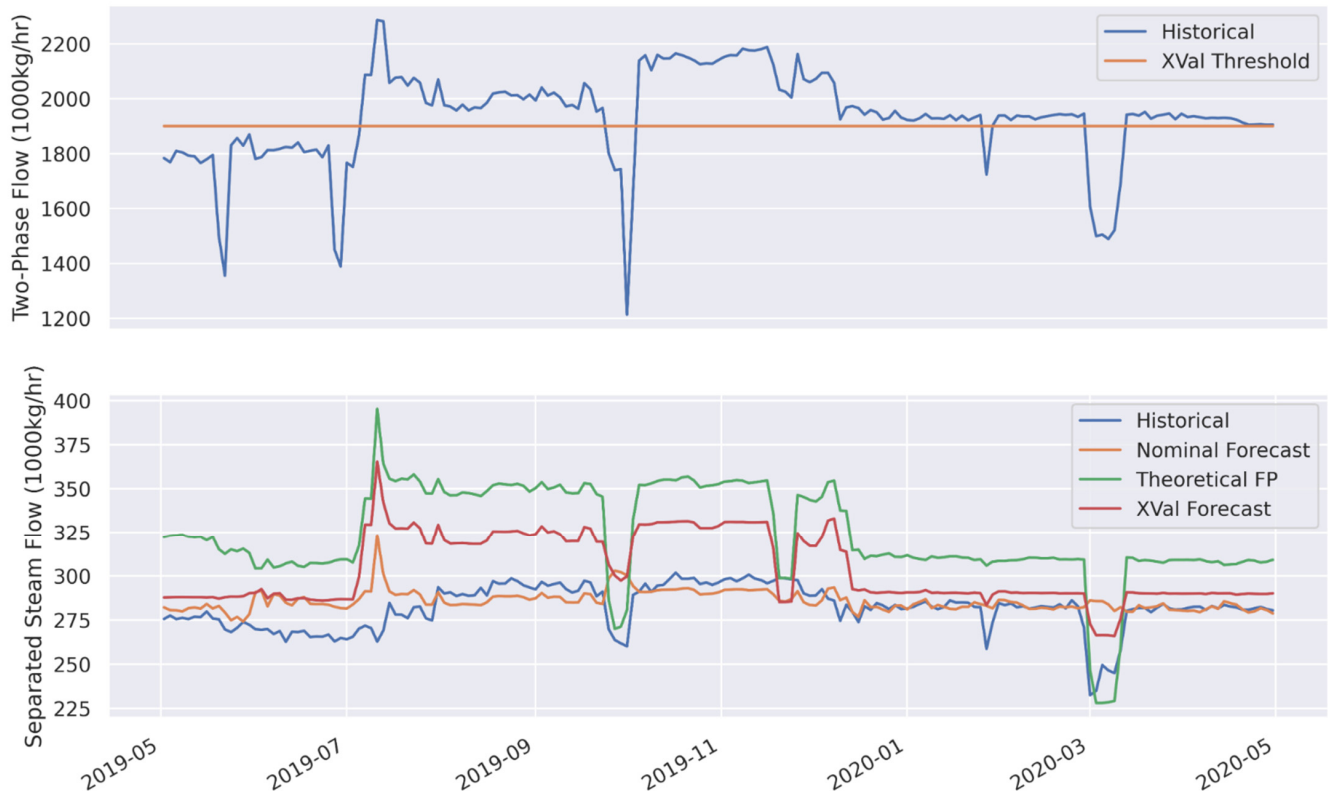
Figure 10. Results from a flash plant modeling cross-validation experiment where models were trained only with two-phase input mass flow less than 1900 tonne/h. The top plot shows the two-phase mass flow through FP16IP+ with the training data limitation. The bottom plot shows the historical separated steam flow compared to predictions by a baseline model trained on all data, the cross-validation (xval) model, and a theoretical model.
