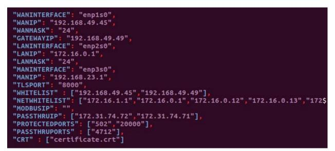
Figure B.8. DERCyST configuration file with 'certificate.crt' in the CRL
