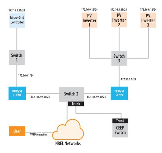
Figure 5. Cyber Range connection to DERCyST testbed
