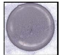
Lithium ring on coin cell electrode
