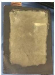
Lithium plating pattern in pouch cell
