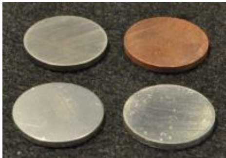
25-mm diameter copper and invar coupons: non-plated (top), plated with 4- \mu m-thick silver (bottom)
