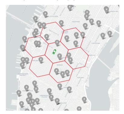
Figure 8. Example of using H3 for a charging station search. The vehicle is seeking a charging location at one of a set of station alternatives, shown as drop points on the map. The search is conducted over an expanding ring of H3 hex grid cells at a higher level of aggregation.
