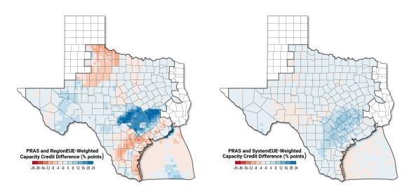
Figure 9. The difference between the CC approximation calculated by the CF weighted by either the Texas system-wide EUE or zone EUE and the Base Case PRAS CC.
