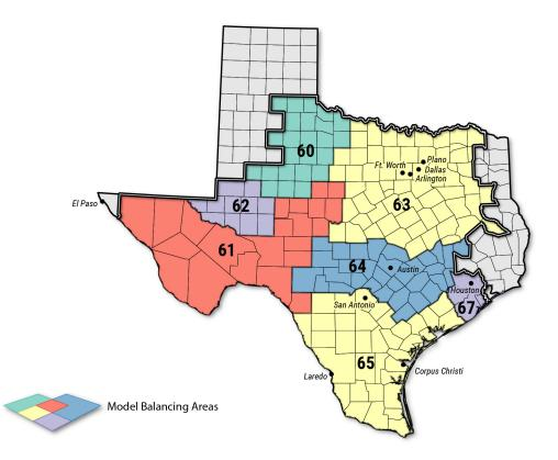
Figure 1. Map of the modeled footprint, including the seven modeled zones with numbers corresponding to the REEDS modeled balancing areas (Brown et al. 2020).
