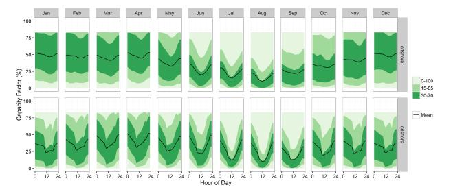
Figure 4. Average diurnal wind CFs from the 7 years of WIND Toolkit data for all grid cells, with ribbons indicating the observed percentiles.
