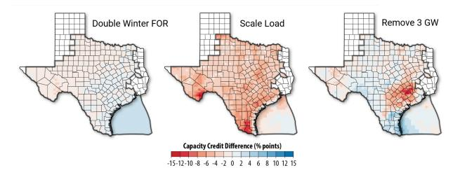
Figure 7. The difference between the Base Case PRAS-computed marginal CC for each grid cell compared to three different variations on the starting PRAS case. A positive indicates the new starting point *increased* the marginal CC, whereas a *negative* value represents a reduced CC.
