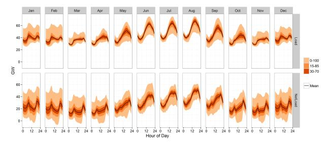
Figure 3. Average diurnal load and net load profiles by month for the Texas Interconnection test system, with ribbons indicating the observed percentiles over the 7 years of data (2007–2013). This reflects our Base Case generator fleet, with 24% generation contribution from wind and 12% from solar.
