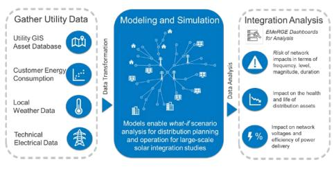
Figure 1. EMeRGE takes key distribution data sets to create holistic models for analysis of the risk to power quality and asset lifetime from the integration of emerging DERs.
