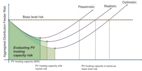
**Figure 3.** EMERGE looks at the risk of emerging DERs, such as solar PV, on utility distribution feeders, allowing planning engineers to make informed planning decisions on DER integration.
