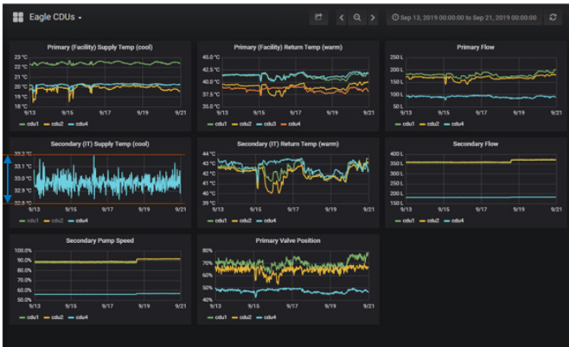
Figure 7: Eagle CDU Dashboard (top row: primary supply temperature, primary return temperature, primary flow; middle row: secondary supply temperature, secondary return temperature, secondary flow; bottom row: secondary pump speed, primary valve position)
