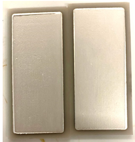
Fig. 2: DBA substrates with screen-printed nano-silver paste during open-faced contact drying on a hot plate. Substrates are 49.2 mm in length by 23.1 mm in width.
