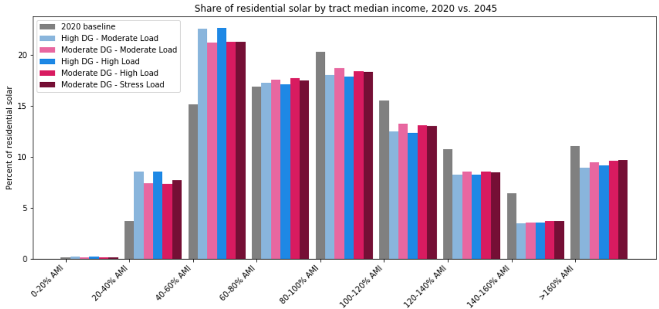
Figure 23. Residential solar adoption share, by tract median income as percentage of area median income and scenario, for census tracts in the city of LA
