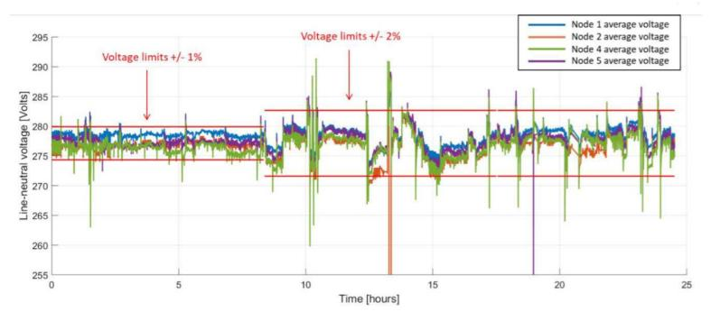
Figure 11. Average line-neutral voltage at nodes in the microgrid
