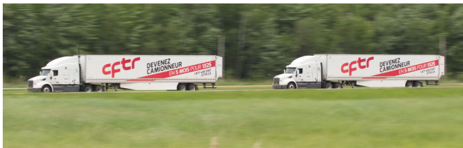
Figure 1. Side-view photograph of Trucks 1 and 2 with 53-ft dry-van trailer and 9 m (30 ft) spacing.
