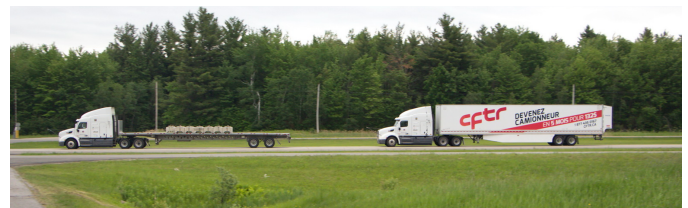
Figure 4. Side-view photograph of Truck 1 with the 53-ft flatbed trailer and Truck 2 with the 53-ft dry-van trailer at 9 m (30 ft) spacing.
