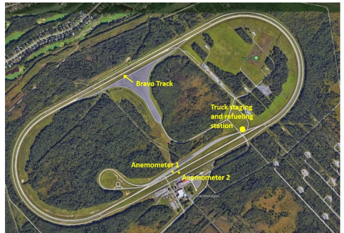
Figure 6. Aerial view of the test track; Location of Track-side anemometers and truck refuelling and staging are shown by yellow circles.
