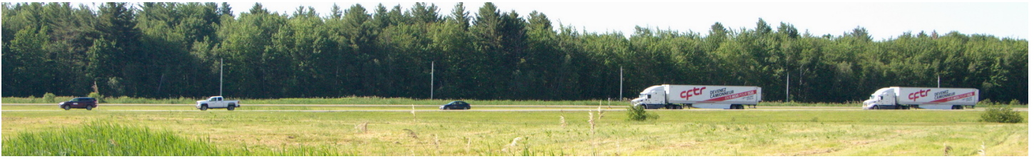
Figure 9. Photograph of the side view of a truck platoon following the light-duty-vehicle traffic pattern.
