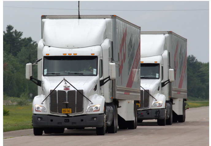
Figure 2. Offset front-view photograph of Trucks 1 and 2 with 53-ft dry-van trailer and 9 m (30 ft) spacing.
