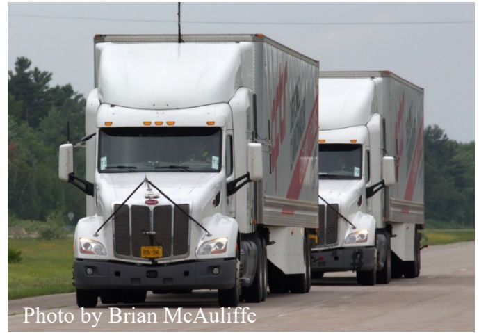
Figure 6: Photograph of Trucks 1 and 2 with 53-ft dry-van trailer and 9 m (30 ft) spacing.
