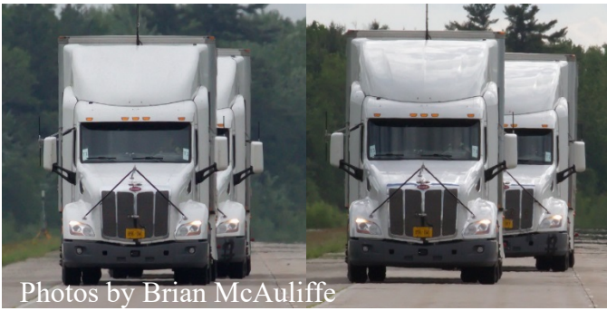
Figure 4: Visual representation of the two offset conditions: left - half offset (0.65 m), right - max offset (1.3 m).
