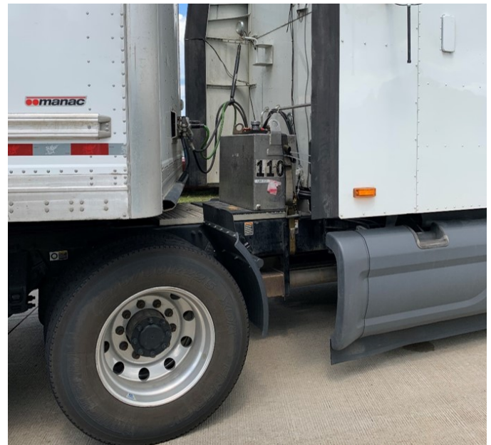
Figure 10: Auxiliary fuel tanks mounted in the tractor-trailer gap.
