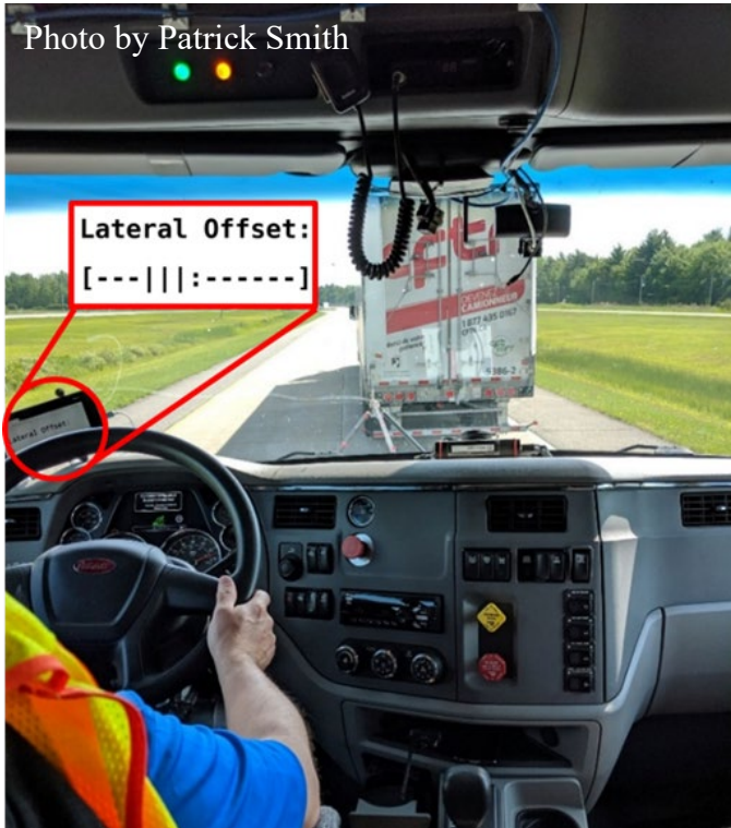
Figure 5: Example test case using the GUI displayed on the tablet (just above steering wheel) for the max offset test case.
