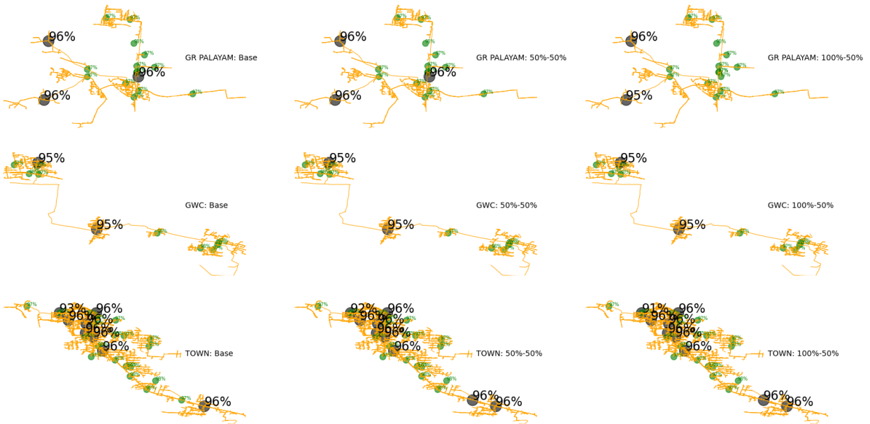
Figure 32. Scatter plot of efficiency of distribution transformers in TANGEDCO feeders in three different PV scenarios ('Base', '50%-50%' and '100%-50%') for 2018
