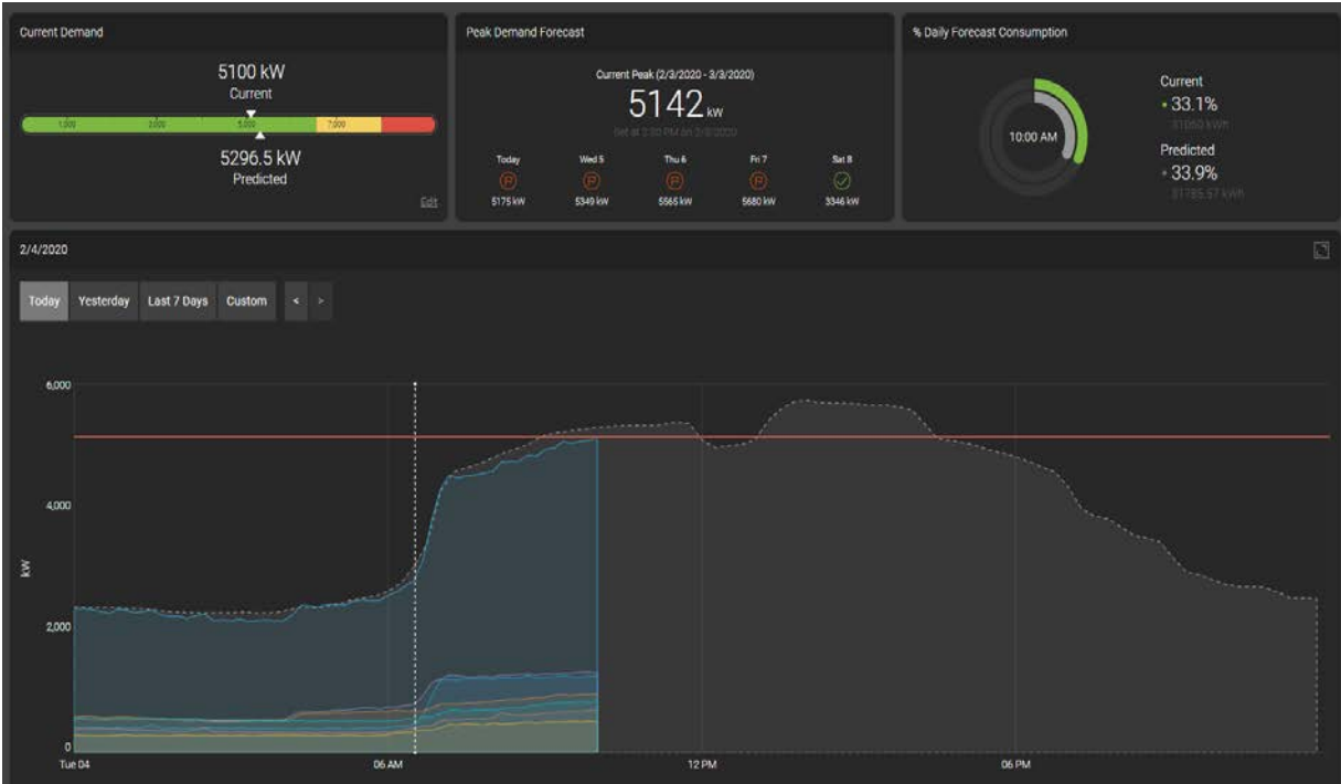
Figure 13. Machine learning model used to predict building load profile over the next 24 hours
