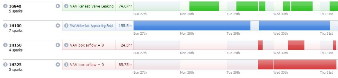
Figure 17. Zone-level fault detection and diagnostics
