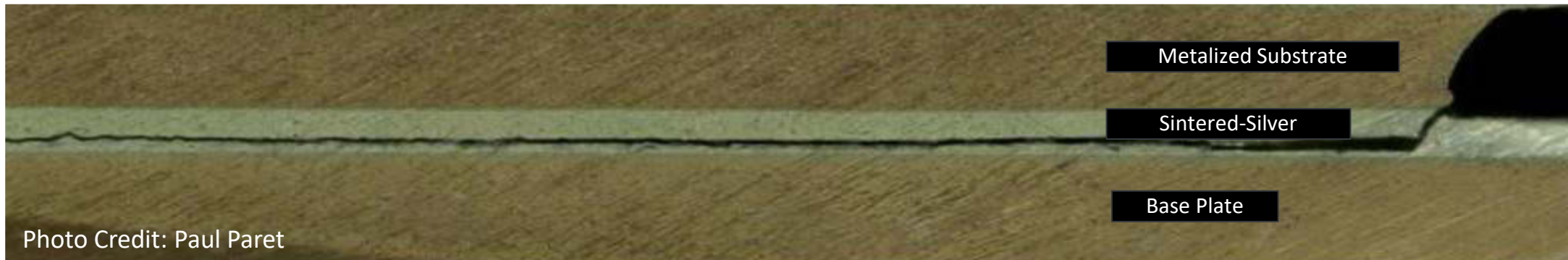
Crack Propagation in Pressure-Assisted Sintered Silver
