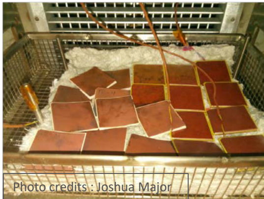
Samples under Thermal Cycling
