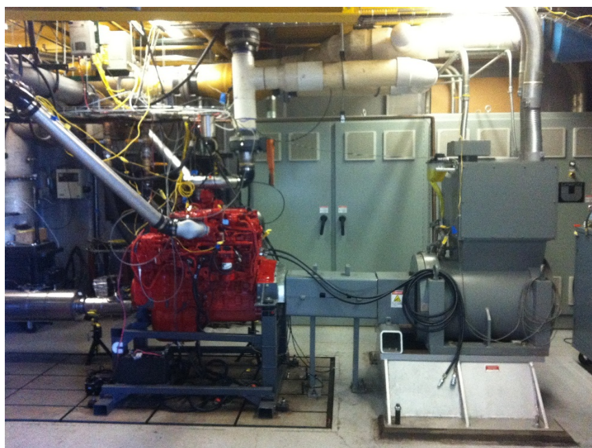
Figure H. 3. Picture of Cummins ISL Diesel Engine in ReFUEL Lab
