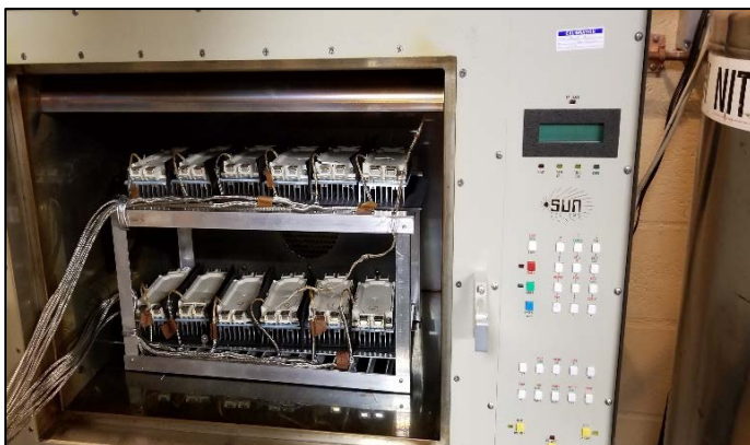
FIGURE 5: SETUP OF POWER MODULES FOR SIMULTANEOUS THERMAL CYCLING.
