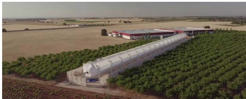
Figure 27. Heliovis inflated HelioTube demonstration in Spain for mushroom drying (Kazkaz 2018). Credit: Heliovis.
