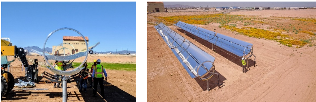
Figure 25. Rackam S20 100-kW th loop being tested at the Heat2Hydro test site in Surprise, Arizona for sludge drying. Photos from Heat2Hydro, credit: Heat2Hydro.
