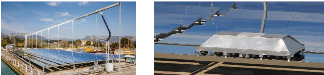
Figure 46: SUNCNIM DSG linear Fresnel collector module (left) and Robotic Cleaning System (right). Photos from SunCNIM, credit SunCNIM.
