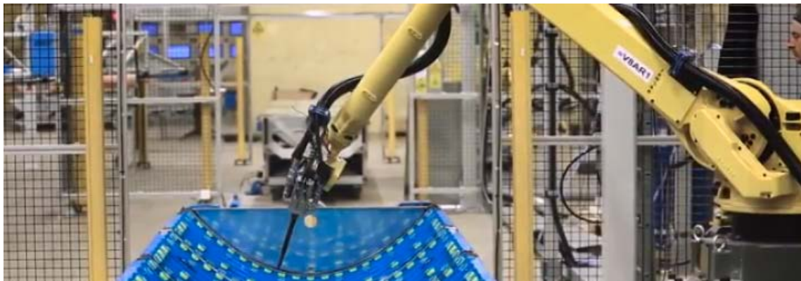
Figure 33. Robotic inspection of Absolicon T160 trough in Swedish manufacturing line (Absolicon 2018a). Credit: Absolicon.
