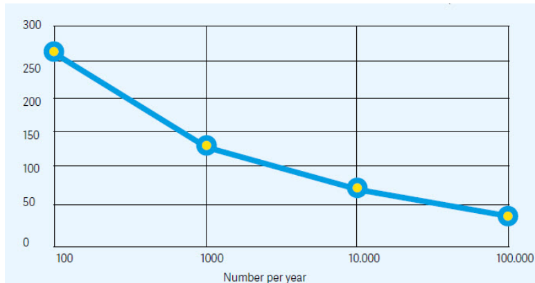
Figure 34. Cost reduction potential (given in SEK) for the Absolicon rear bulkhead through mass manufacturing investments (Absolicon 2018c).
