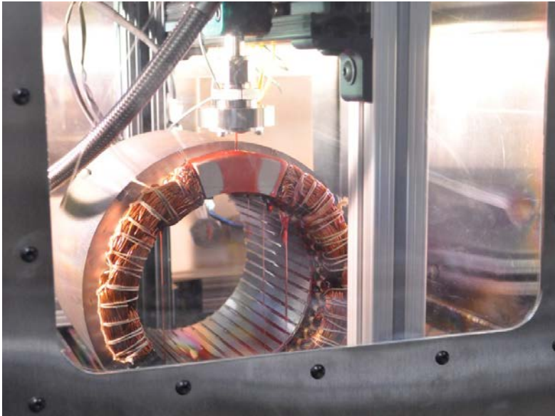
Direct Cooling of Motor Windings
