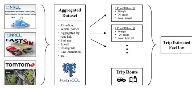
FIGURE 1 From left to right: the data pre-processing and powertrain simulation steps, the results of which are aggregated into a large data set from which an energy estimation look-up table for that particular vehicle model can be generated. Trip fuel use is estimated by combining the model results with a proposed trip route.
