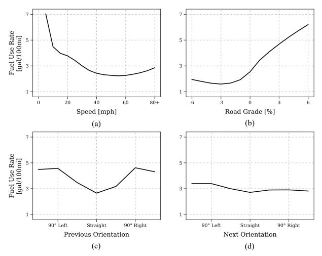
FIGURE 2 Driving and road network attributes plotted against vehicle fuel use rate for a conventional vehicle to determine the most important attributes to include in the energy estimation model. (a) Vehicle average speed over a pass vs. fuel use rate, (b) link average road grade vs. fuel use rate, (c) severity of turn from the previous link to the current vs. fuel use rate on the current link, and (d) severity of turn from the current link to the next link vs. fuel use rate on the current link.
