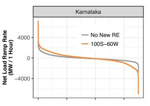
Peak I-hour net load up-ramp in the 100S-60W scenario is 7.3 GW, up from 3.3 GW in the No New RE scenario. Maximum net load valley-to-peak ramp is 10 GW in the 100S-60W scenario, up from 6.2 GW in the No New RE scenario.
