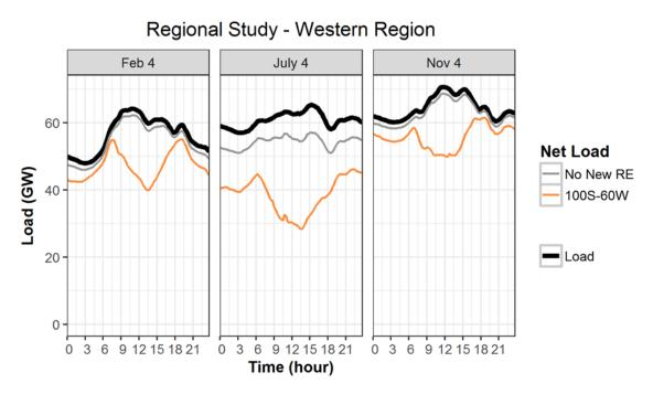
Figure 24. Comparison of net load by season, No New RE and 100S-60W, Western region Net load is load minus wind and solar generation post-curtailment.
