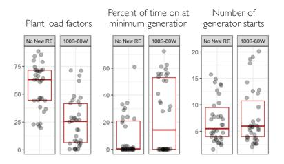
While coal PLFs are lower fleetwide in 100S-60VV, generators with higher variable costs are impacted more.
