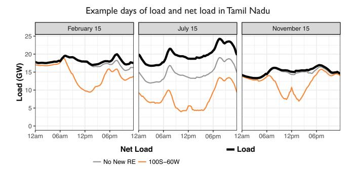
Increased daytime solar generation causes a dip in net load, which requires Tamil Nadu to either increase net exports, turn down its thermal generators, or curtail RE. On 15 July, increased monsoon season wind generation reduces Tamil Nadu's net load throughout the day.
