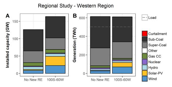
Figure 21. Installed capacity (A) and annual generation (B), No New RE and 100S-60W, Western region
