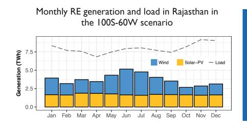
solar produce 49% of total generation in Rajasthan and meet 47% of load.
