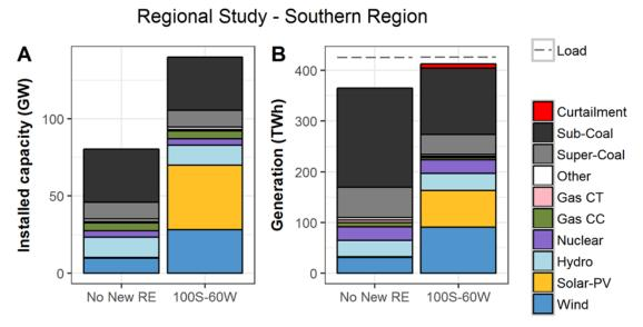
Figure 3. Installed capacity (A) and annual generation (B), No New RE and 100S-60W, Southern region
