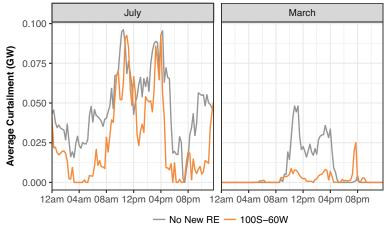
Maharashtra experiences the lowest RE curtailment of any state with significant RE capacity. Its thermal fleet is fully constrained only 0.2% of the year in the 100S-60VV scenario, indicating that the RE curtailment that does happen is caused primarily by transmission congestion and trade barriers.
