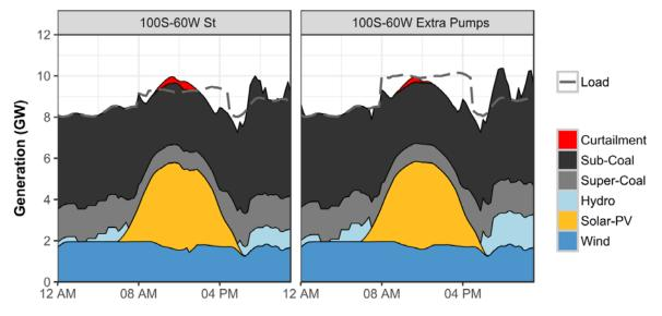
Figure 45. Comparison of dispatch in Telangana on 20 June, with and without extra pumps
