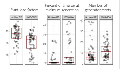
While coal PLFs are lower fleetwide in 100S-60W, the most expensive generators experience the greatest drop in PLF. Average PLF of coal generators in Gujarat, disaggregated by variable cost
