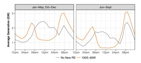
Minimum generation limits and higher hydro energy availability during the nonmonsoon season hinder the ability of hydro to shift generation to net load peaks as it does more fully in June through September.
