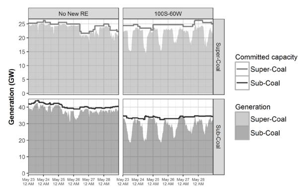
Figure 27. Committed capacity and generation during a high-RE week, 23–29 May, for sub- and supercritical coal, No New RE and 100S-60W, Western region
