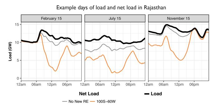
Increased daytime solar generation causes a dip in net load, which requires Rajasthan to either increase net exports, turn down its thermal generators, or curtail RE. On 15 July, increased monsoon season wind generation shifts Rajasthan's net load curve downward during all hours of the day.
