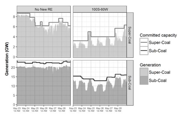
Figure 9. Committed capacity and generation during a high-RE week, 23–29 May, for sub- and supercritical coal, No New RE and 100S-60W, Southern region
