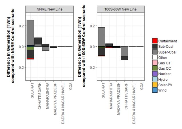
Figure 42. Difference in generation with the new line compared to the control scenario in the Western region by state, No New RE and 100S-60W
