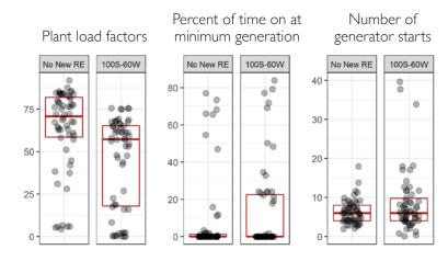
While coal PLFs are lower fleetwide in 100S-60VV, the most expensive generators experience the greatest drop in PLF. Average PLF of coal generators in Tamil Nadu, disaggregated by variable cost
