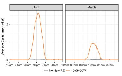
Karnataka experiences the highest RE curtailment as a percent of available capacity in the Southern region, particularly in October and November when curtailment exceeds 18%. It has the lowest ratio of thermal to RE capacity in the region, making curtailment sensitive to minimum coal generation levels, transmission constraints, and trade barriers.
