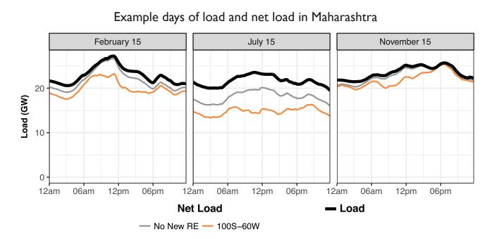
Because of its large size and high wind capacity relative to solar in the 100S-60W scenario, Maharashtra experiences less severe daytime net load ramps than other high-RE states. Its load often peaks midday, as on 15 February and 15 July, during which solar generation smooths the net load profile.
