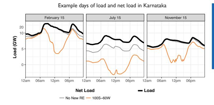
Increased daytime solar generation causes a dip in net load, which requires Karnataka to either increase net exports, turn down its thermal generators, or curtail RE. On 15 July, increased monsoon season wind generation drives Karnataka's daytime net load below zero (>100% RE penetration) for several hours. However, despite its lower RE penetration, 15 November has the larger nationwide valley-to-peak net load ramp, and RE curtailment on that day is higher.
