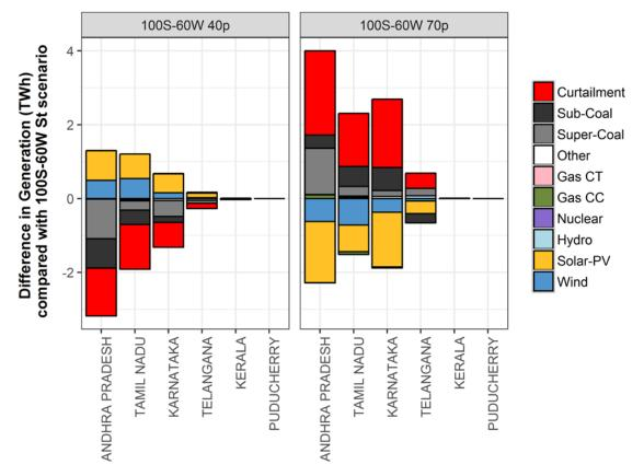
Figure 15. Difference in generation in lower and higher minimum generation levels compared to the base case of 55%, in the Southern region by state
