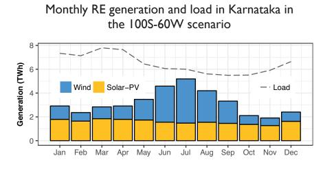
solar produce 48% of total generation in Karnataka and meet 49% of load.
