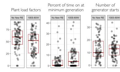
While coal PLFs are lower fleetwide in 100S-60VV, the most expensive generators experience the greatest drop in PLF. Average PLF of coal generators in Maharashtra, disaggregated by variable cost
