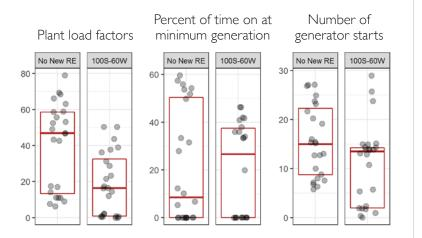
Coal plant load factors (PLFs) are lower in the 100S-60W scenario due to more frequent cycling and operation at minimum generation levels.
