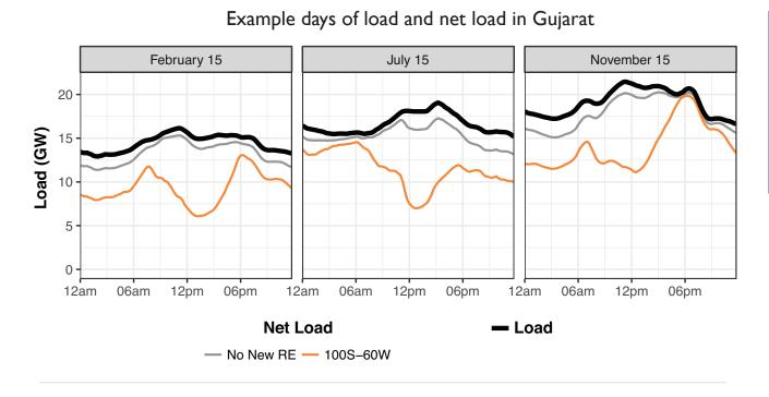
Increased daytime solar generation causes a dip in net load, which requires Gujarat to either increase net exports, turn down its thermal generators, or curtail RE.
