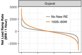
Peak I-hour net load up-ramp in the I00S-60W scenario is 4.7 GW, up from 2.7 GW in the No New RE scenario. Maximum net load valley-to-peak ramp is 12 GW in the 100S-60W scenario, up from 6.9 GW in the No New RE scenario.
