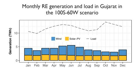
Wind and solar produce 35% of total generation in Gujarat and meet 35% of load.
