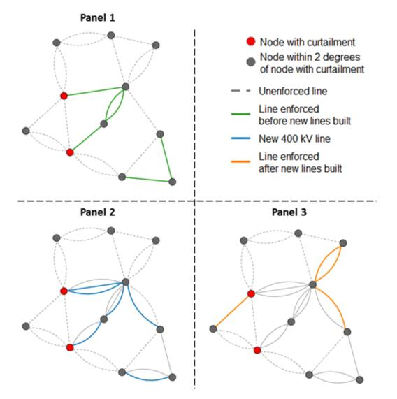
Figure 49. Example of the iterative process of adding and enforcing lines in a small section of the Rajasthan network
