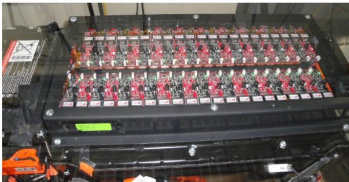
Figure 4. Ford C-Max PHEV battery pack with prototype DC/DC converters
