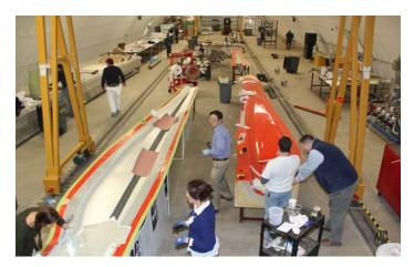
The Composites Manufacturing Education and Technology facility expedites manufacturing by enabling researchers to design, prototype, test, and manufacture composite wind turbine blades and other components in one location. *Photo by David Snowberg, NREL/41769*
