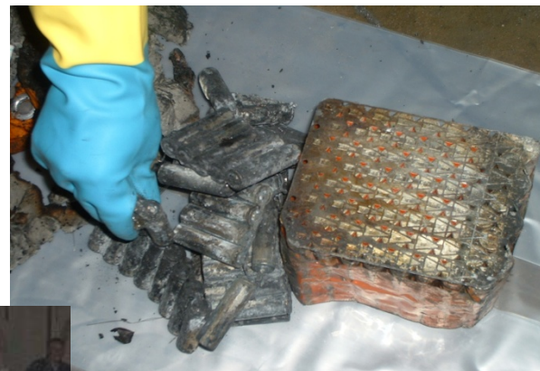
Aftermath of an external short incident
