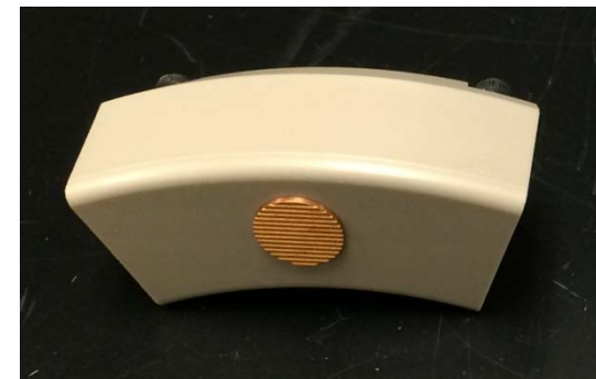
Assembled test fixture for end-surface heat transfer measurement
