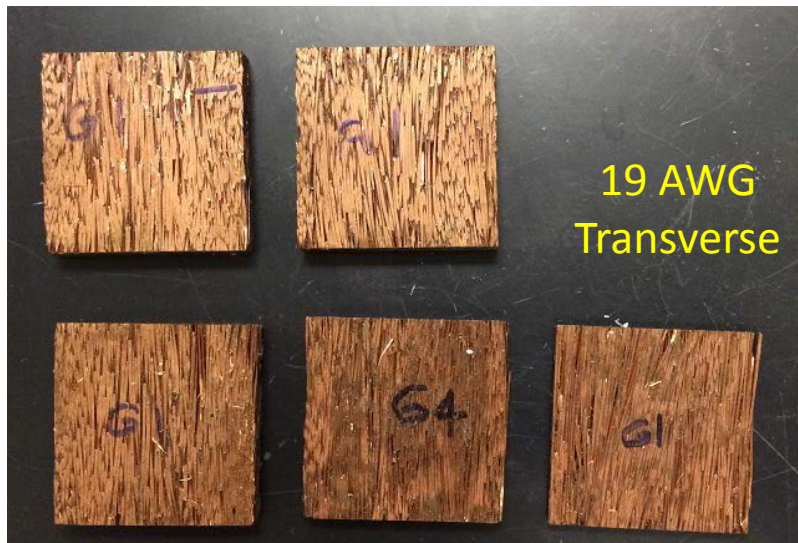
Winding sample blocks prepared by ORNL
