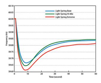
energy storage were examined, and limited application was effective at improving frequency response. Refinements to these controls would further improve performance.
