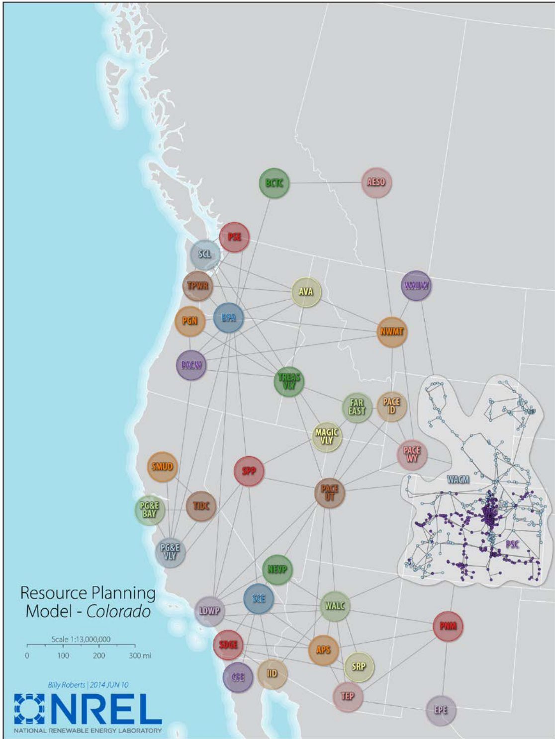
Figure 1. Combined zonal/nodal structure used for the CO-centric version of RPM
