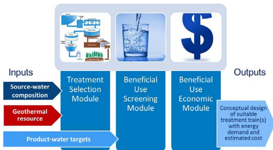
Figure 3. Conceptual framework for selecting a treatment train. Modifications to the pre-existing CSM decision support tool are highlighted in green.
